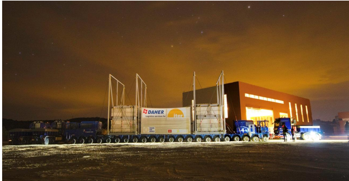
2 nd Test Convoy in April 2014 Heavy Component on Road (TF Coils, VV Sectors, and PF1 Coil)
