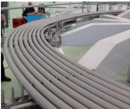
Fig.1 Wound conductors before heat treatment and insertion into radial plates
