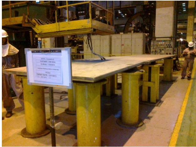
Cryostat pedestal ring - top plate 200 mm and skirt plate 105 mm thick welded together
