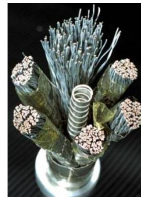
Fig. 5 Cable in conduit made of 900 Nb 3 Sn strands in multistages with central channel into 316LN jacket
