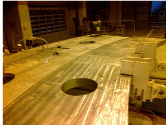
Cryostat pedestal ring - top plate 200 mm and skirt plate 105 mm thick welded together
