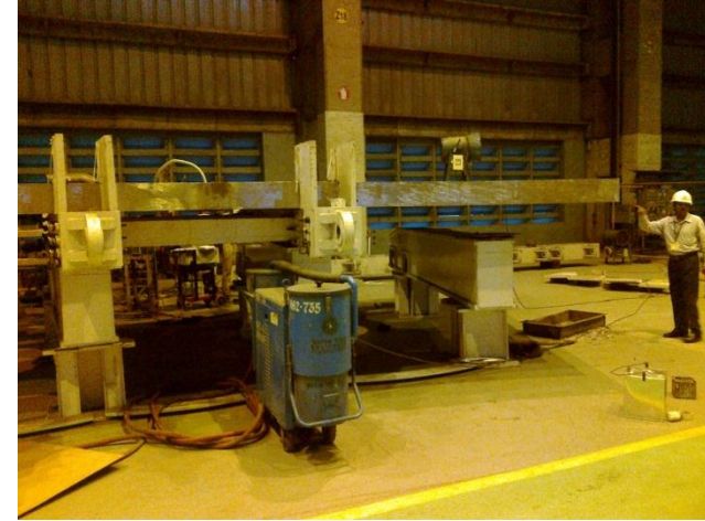
Cryostat pedestal ring - top plate 200 mm and skirt plate 105 mm thick welded together
